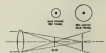
FIG. 1—Since refractivity of glass is greater for blue than for red, blue light will focus at a point near the lens than will red.
